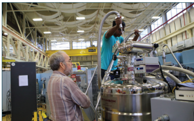
Scott Dewey (NCNR) supervising Ripan Biswas (Tulane University) as he replenishes liquid Helium for the neutron lifetime experiment at NG-C.
