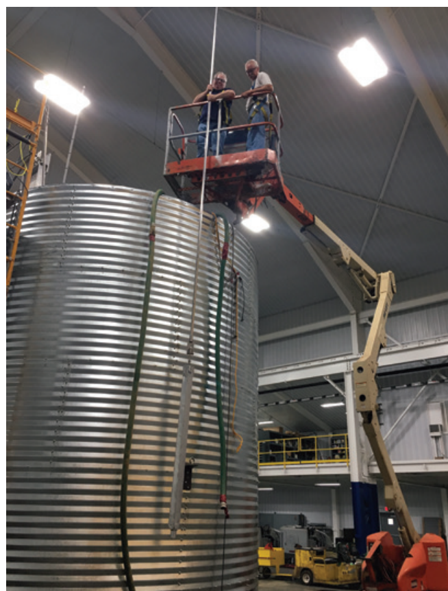
FIGURE 2: Fuel saw assembly submerged in test tank, which was designed to mimic the storage pool. Scott Slaughter is handling a dummy fuel element.
