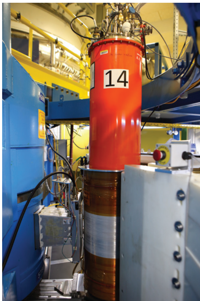
FIGURE 5: The integrated polarized MACS setup with the newly developed dedicated cryostat is being tested for safe and reliable operation and performance evaluation on MACS.
