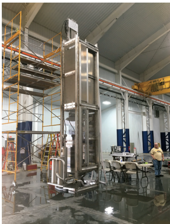
FIGURE 1: Fuel saw assembly with Scott Slaughter looking on. The chip management system is on the left front side.
