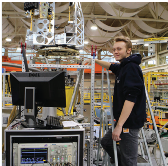
Tim Reeder from the Institute for Quantum Matter at Johns Hopkins University installing a microwave device on the 10 T magnet in preparation for a MACS experiment.
