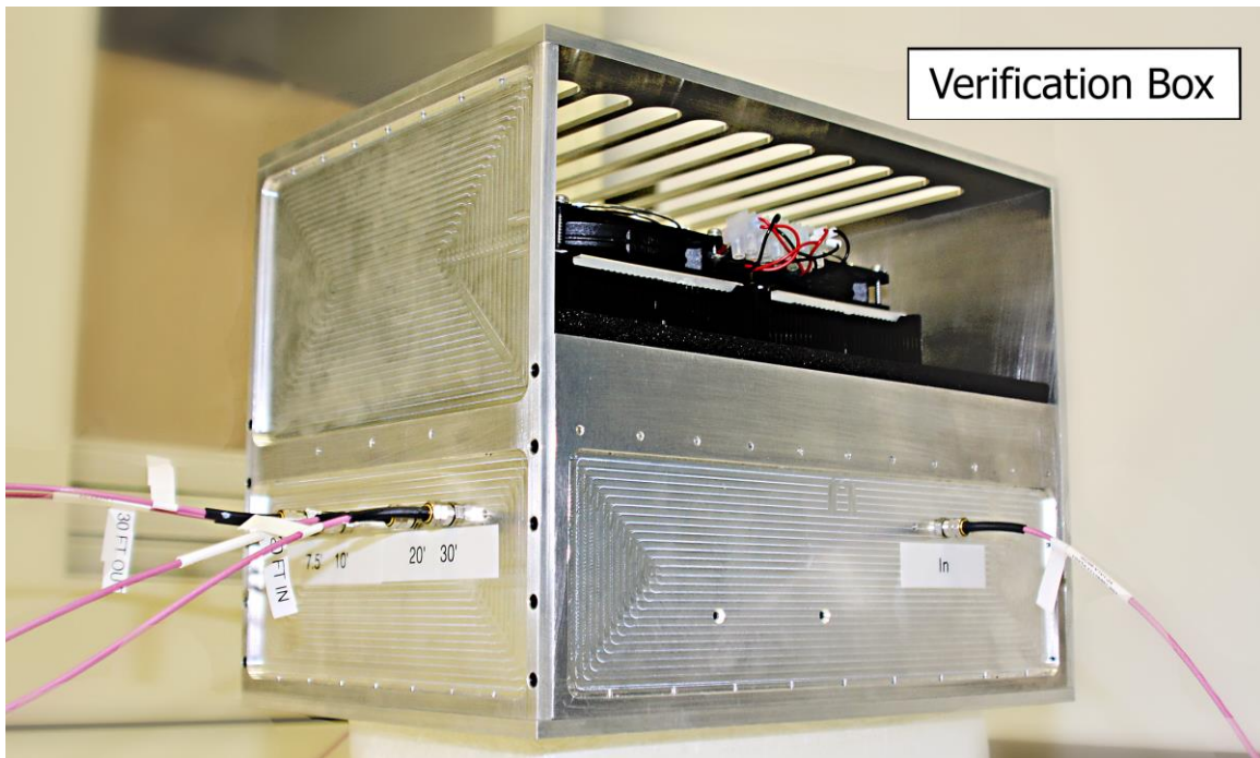
Fig. 1: The temperature-controlled NIST channel sounder verification box. The box dimensions are approximately 210 x 240 x 300 cm 3 .
