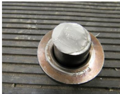
Fig. 4: shear rupture in bolt (SP005)
