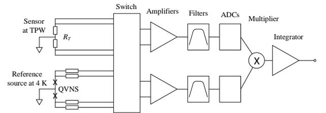
**Figure 4:** The QVNS thermometer. When measuring the Boltzmann constant, the thermal sensor is maintained at the triple point of water.
