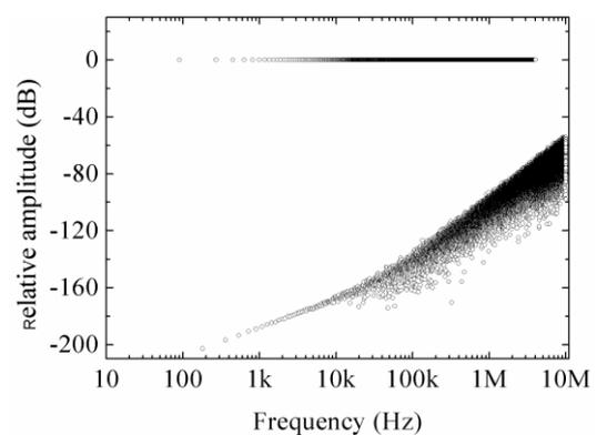
**Figure 3.** The QVNS spectrum calculated from the QVNS code sequence. The upper branch shows the odd harmonics and the lower branch shows the even harmonics. The amplitudes of the even harmonics are indicative of the variation of the amplitudes of the odd harmonics from the target voltage.
