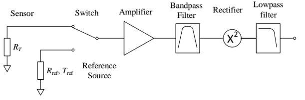
**Figure 1.** A simplified schematic diagram of a switched-rectifier Johnson noise thermometer.
