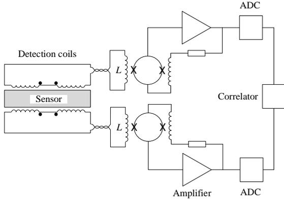
**Figure 7.** Schematic of a cross-correlating current-sensing noise thermometer with gradiometer (differential) sensing coils.
