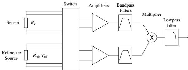
**Figure 2.** A simplified schematic diagram of the switched-correlator noise thermometer.
