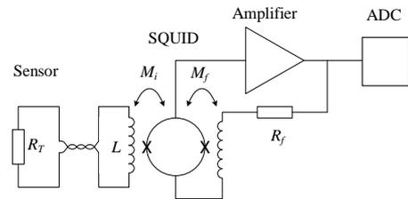
**Figure 6.** The current-sensing noise thermometer.
