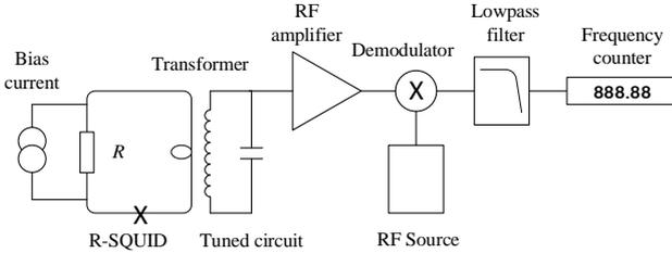
**Figure 5.** Schematic diagram of the R-SQUID noise thermometer
