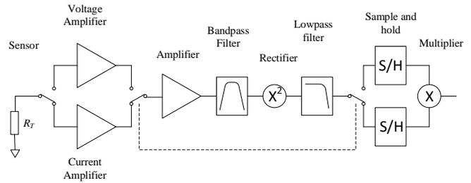
**Figure 13.** The noise-power thermometer measures the product of the noise current and the noise voltage.
