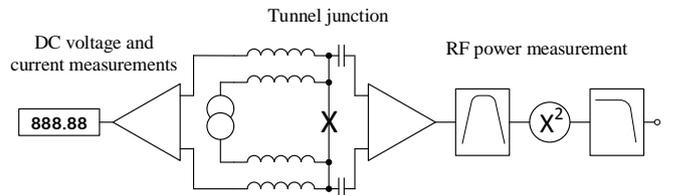
**Figure 10.** Schematic diagram of the shot noise thermometer.
