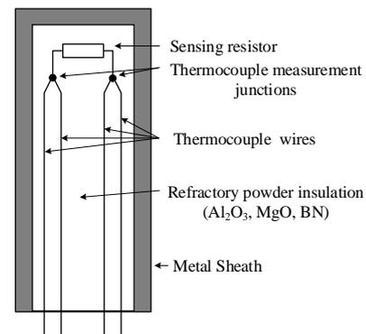
Figure 12. Combined noise-thermocouple sensor.
