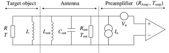
**Figure 15.** Equivalent circuit for the inductive noise thermometer.
