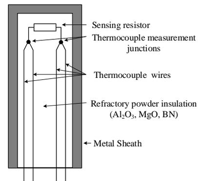
**Figure 12.** Combined noise-thermocouple sensor.
