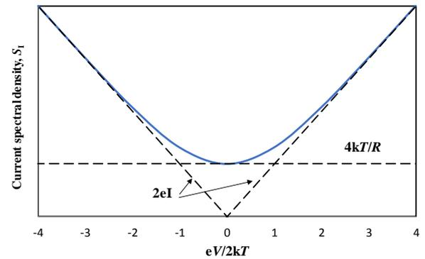
**Figure 9.** Normalised plot of the spectral density of the tunnel junction shot noise versus bias voltage showing the limiting behaviours for small and large bias voltages.
