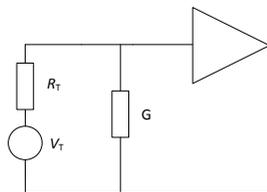
**Figure 19.** simplified model of the effect of poor electrical insulation at high temperatures.
