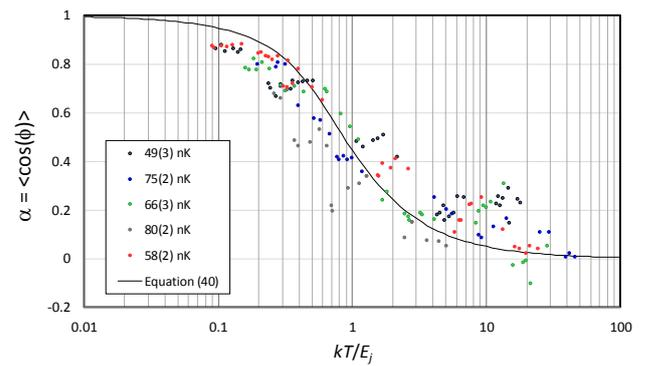
**Figure 11.** The measured coherence factor versus normalised energy for the bosonic junction thermometer, compared with theory. The scatter is due to the small number of measurements made for each point.
