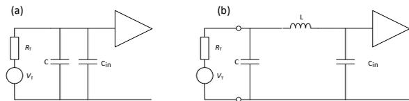
**Figure 18.** a simplified models (a) first order in frequency, (b) third-order in frequency.
