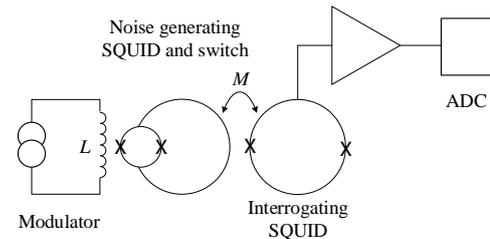
**Figure 8.** The quantum-roulette noise thermometer. The modulator switches the Josephson junctions between superconducting and normal states.
