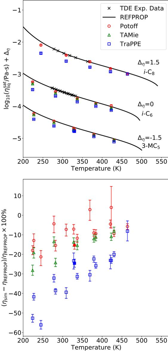
Figure 5: Saturated liquid viscosities for 2-methylpentane ( $i\text{-C}_6$ ), 3-methylpentane ( $3\text{-MC}_5$ ), and 2,2,4-trimethylpentane ( $i\text{-C}_8$ ). See Figure 1 caption for details. For clarity, values in top panel are shifted by  $\Delta\eta$ . Filled symbols correspond to simulations performed at the respective force field  $\rho_{\text{liq}}^{\text{sat}}$  (see Section 4).
