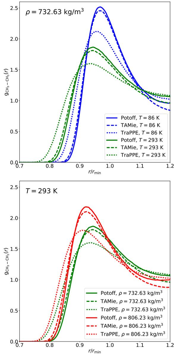
Figure 13: Comparison of radial distribution functions for  $\text{CH}_3\text{-CH}_3$  interactions ( $g_{\text{CH}_3-\text{CH}_3}(r)$ ). The top panel compares two different temperatures along the triple point isochore. The bottom panel compares two different densities along the 293 K isotherm. Colors correspond to different state points while line styles denote different force fields.
