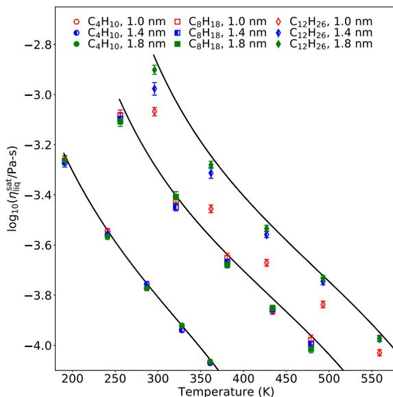
Figure 15: Impact of cut-off distance. Colors/symbols denote different cut-off lengths. Different shapes correspond to *n*-butane, *n*-octane, and *n*-dodecane. REFPROP values are provided as lines for visual reference. Simulations are performed with Potoff force field at saturation conditions.
