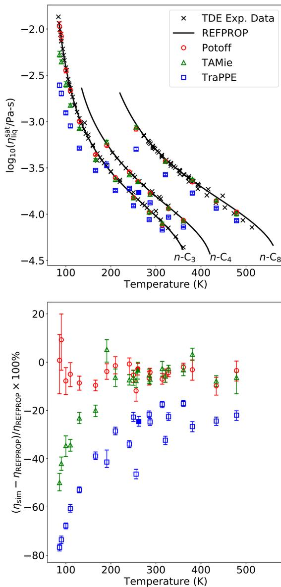
Figure 2: Saturated liquid viscosities for propane ( $n\text{-C}_3$ ),  $n$ -butane ( $n\text{-C}_4$ ), and  $n$ -octane ( $n\text{-C}_8$ ). See Figure 1 caption for details. Filled symbols correspond to simulations performed at the respective force field  $\rho_{\text{liq}}^{\text{sat}}$  (see Section 4).
