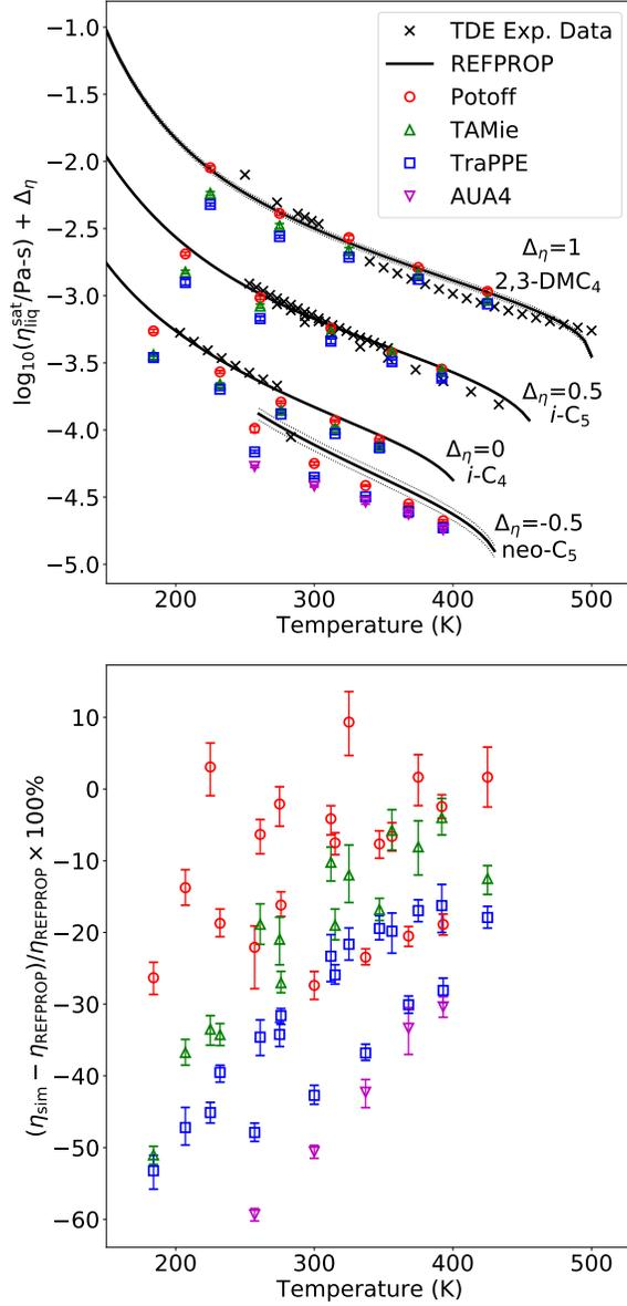
Figure 4: Saturated liquid viscosities for 2-methylpropane (*i*-C<sub>4</sub>), 2,2-dimethylpropane (neo-C<sub>5</sub>), 2-methylbutane (*i*-C<sub>5</sub>), and 2,3-dimethylbutane (2,3-DMC<sub>4</sub>). See Figure 1 caption for details. For clarity, values in top panel are shifted by  $\Delta\eta$ .
