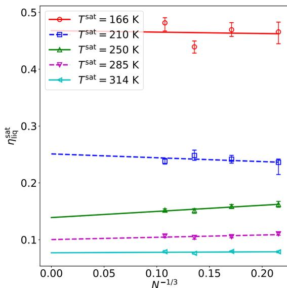
Figure 14: Finite-size effects. Simulation results were obtained for propane with the Potoff force field and  $N = 100, 200, 400,$  and  $800$ . Colors/symbols denote different saturation temperatures. The lines are obtained from a weighted linear fit with respect to  $N^{-1/3}$ .
