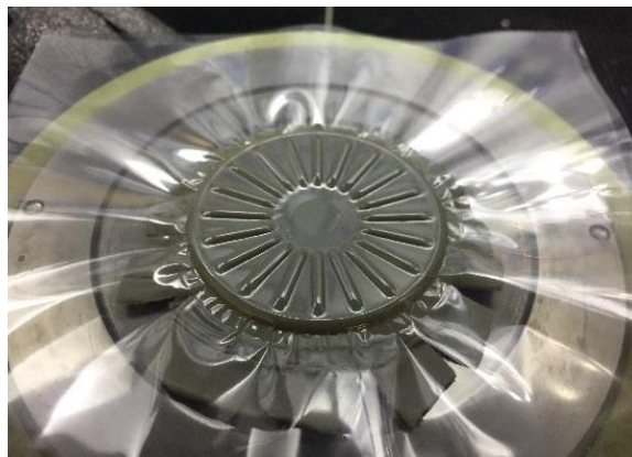
Figure 1. Test specimen (Roma Plastilina No. 1) is placed between two sheets of polyester film for rheological tests using rubber process analyzer. The image shows the specimen in a pressed form after the test is done.
