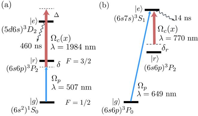
FIG. 3. (a) Atomic levels for the blue- and red-detuned ac-Stark schemes in  $^{171}\text{Yb}$ . (b) Atomic levels for the EIT scheme in bosonic Yb atoms. In all schemes, the main limitation comes from the admixture of levels outside the three-level system.
