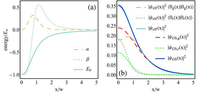
FIG. 2. Analysis of the blue-detuned ac-Stark scheme [Fig. 1(b)]. (a) The light shift  $E_0(x)$ , as well as the diagonal and off-diagonal couplings coming from the nonadiabatic potential  $U$  in Eq. (7) parametrized by  $\alpha$  and  $\beta$ . (b) Properties of the ground state obtained from the effective Hamiltonian and from the full Hamiltonian (see main text for details). Figures are shown in units of  $w$  and  $E_w$ , making them applicable to all  $s \gg 1$ .
