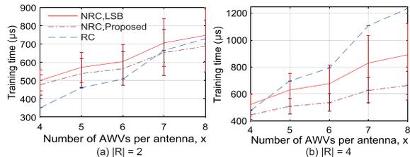
Fig. 6. Training time of the MIMO phase for 1000 simulations.
