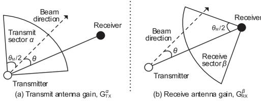
Fig. 4. Example of the azimuth angles for (a)  $G_{TX}^{\alpha}$  and (b)  $G_{RX}^{\beta}$ .
