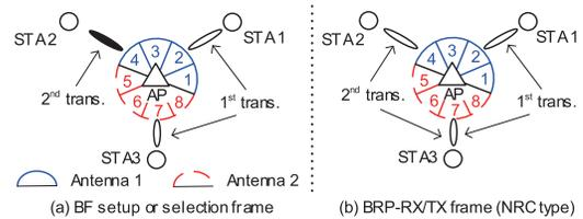
Fig. 3. Example of transmit antenna configuration in the MIMO phase.
