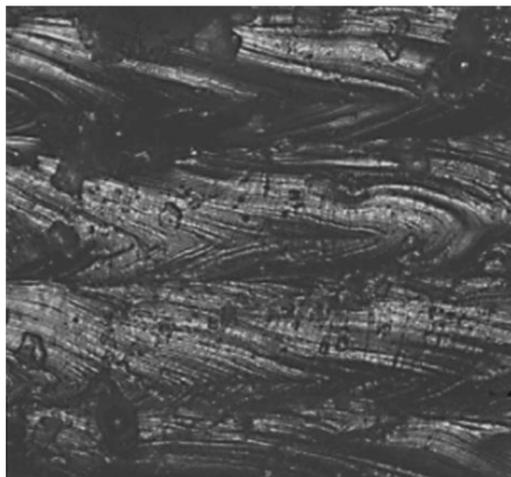
Figure 2. Chevron pattern on upward facing surface of AM part
