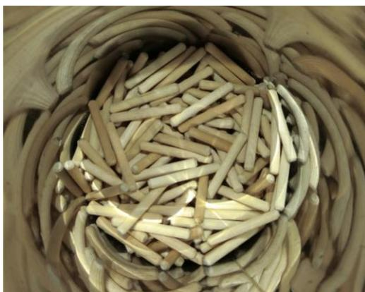
**Figure 7** Fuel batch loaded in firebrand generator
