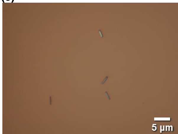
Figure S20. Additional optical microscopy images taken from both concentrated regions (a,b,d) and dilute regions (c,e,f) of drop-cast \mu\text{m} -scale 2D SnS nanoribbons (left column) and square nanosheets (right column).
