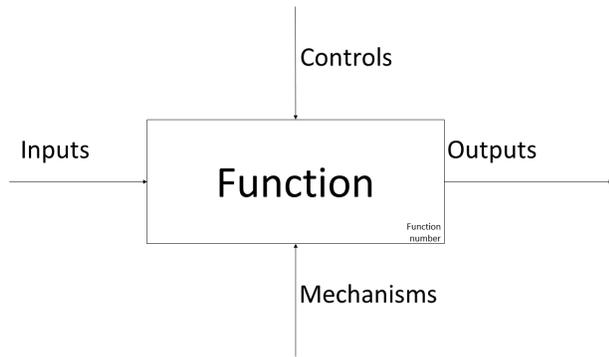
Fig. 2. IDEF0 diagram: boxes represent functions, arrows represent inputs, outputs, controls, and mechanisms as described in [42].
