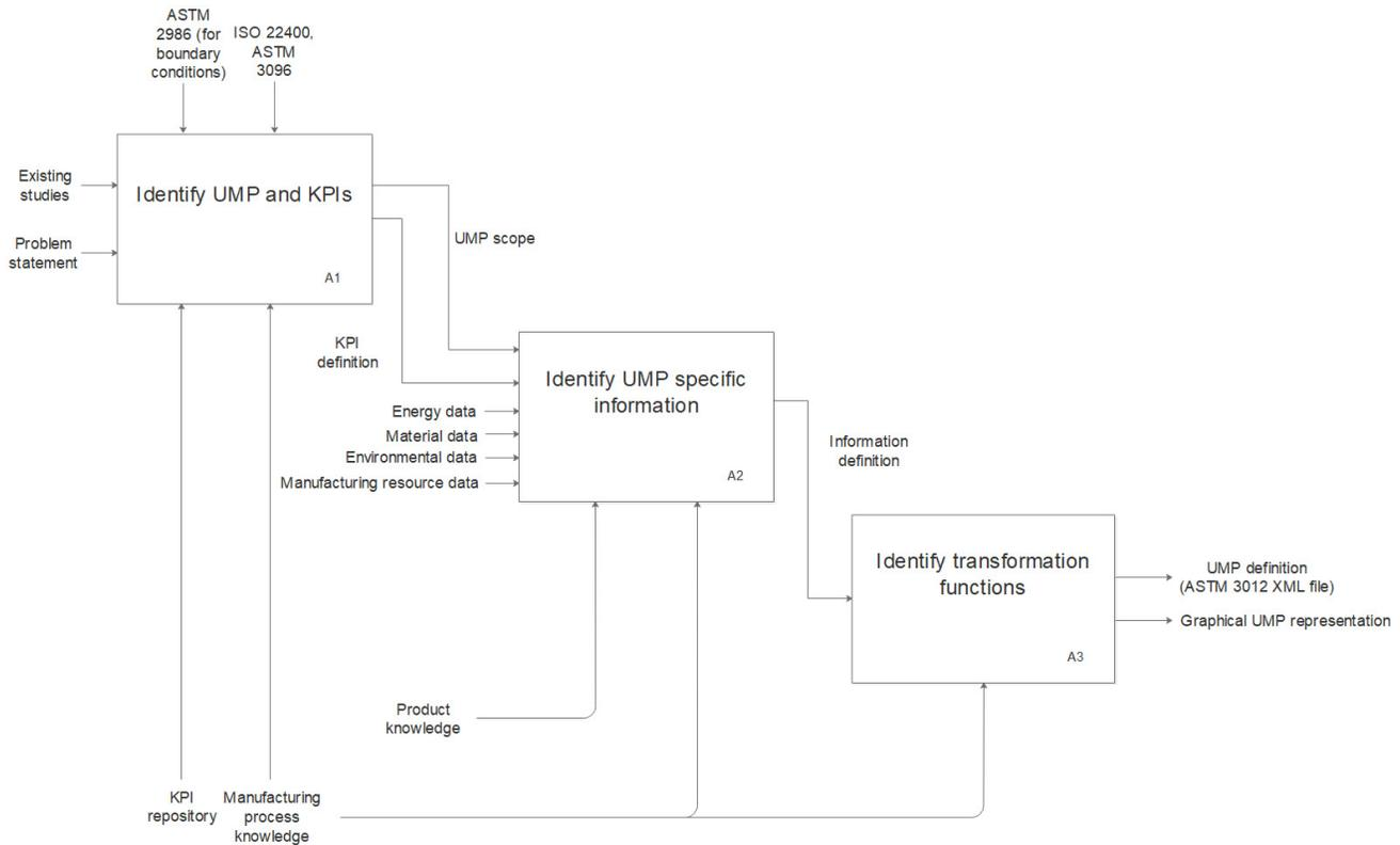
Fig. 4. IDEFO diagram describing activities for Environmental characterization of manufacturing processes.
