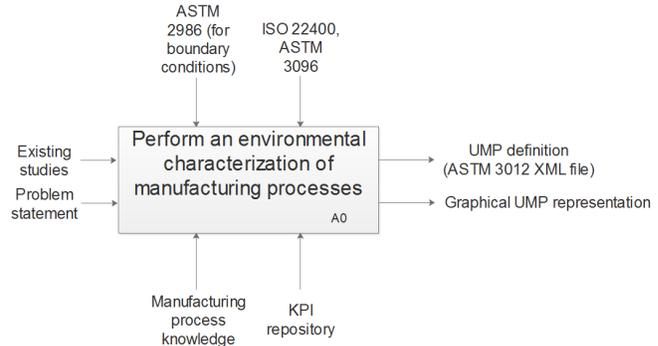
Fig. 3. The IDEF0 diagram for performing activity A0: Environmental characterization of manufacturing processes.
