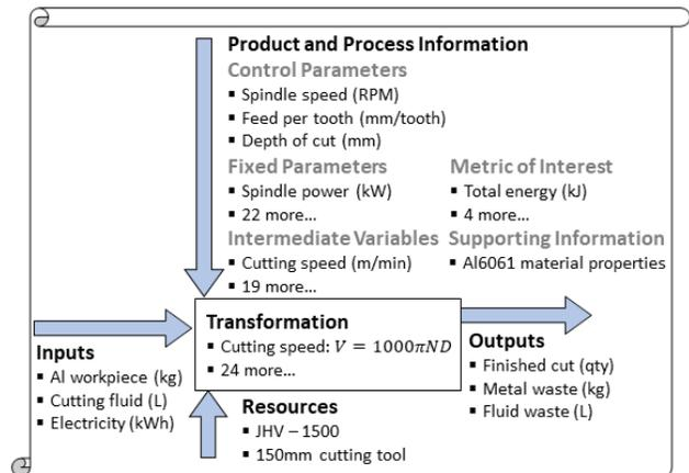
Fig. 11. ASTM E3012 graphical representation of the milling UMP.
