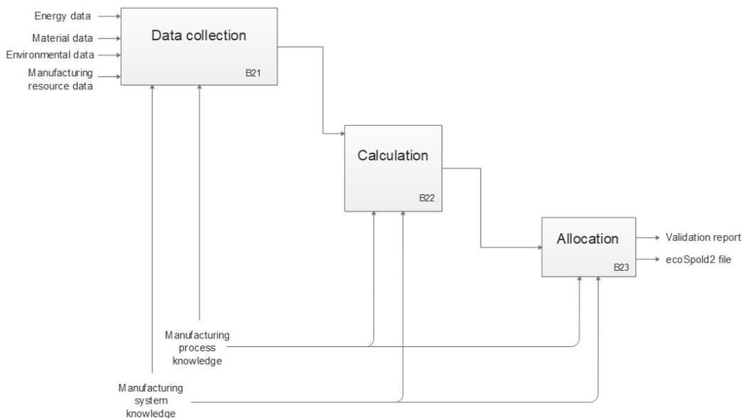
Fig. 8. IDEF0 diagram describing subactivities for running an inventory analysis.
