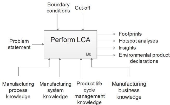
Fig. 6. The IDEF0 diagram for performing activity B0: Perform LCA.
