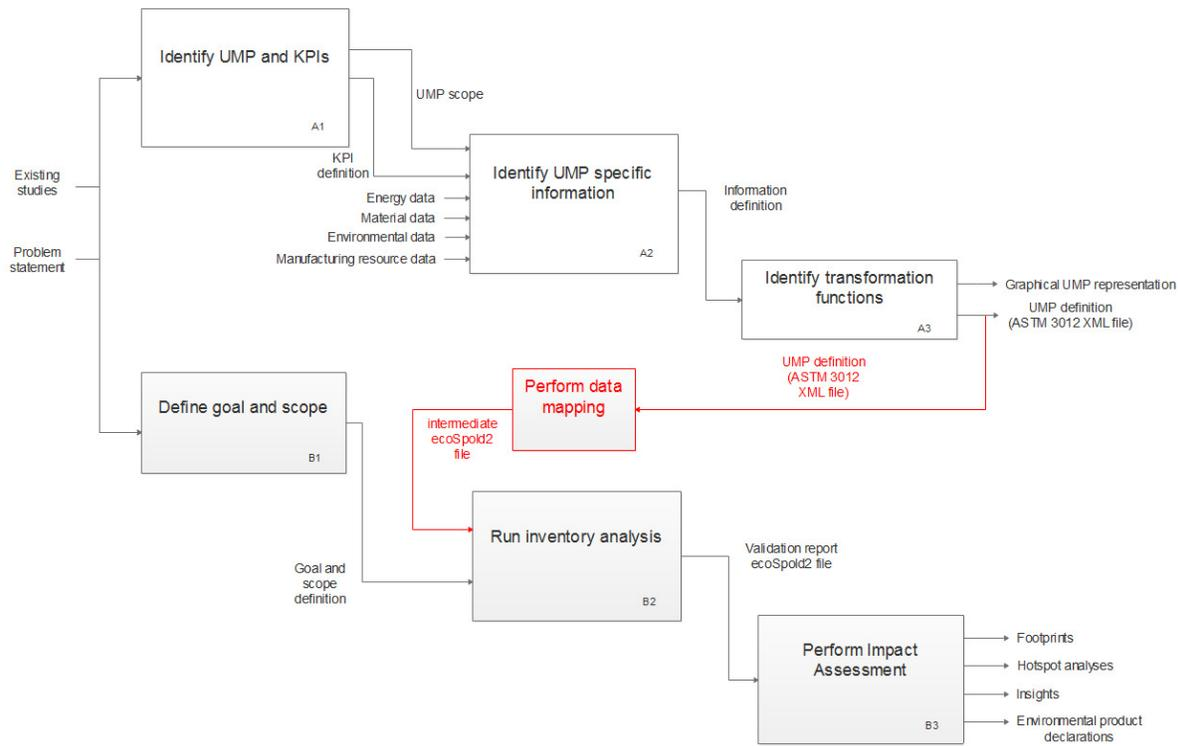
Fig. 9. IDEF0 diagram describing activities for creating LCI data using the UMP format.
