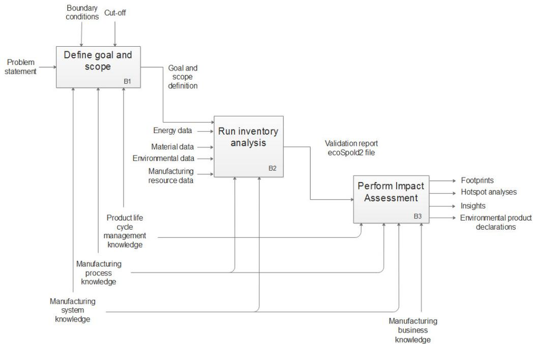
Fig. 7. IDEF0 diagram describing activities for an LCA.
