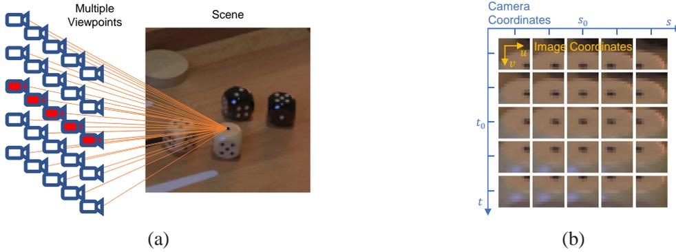
Fig 1: Light field imaging. (a) A scene observed from multiple viewpoints in a light field camera and (b) the subimages from multiple viewpoints and the camera and image coordinates. Source of the light field image: 4-D Light Field Benchmark.<sup>7</sup>
