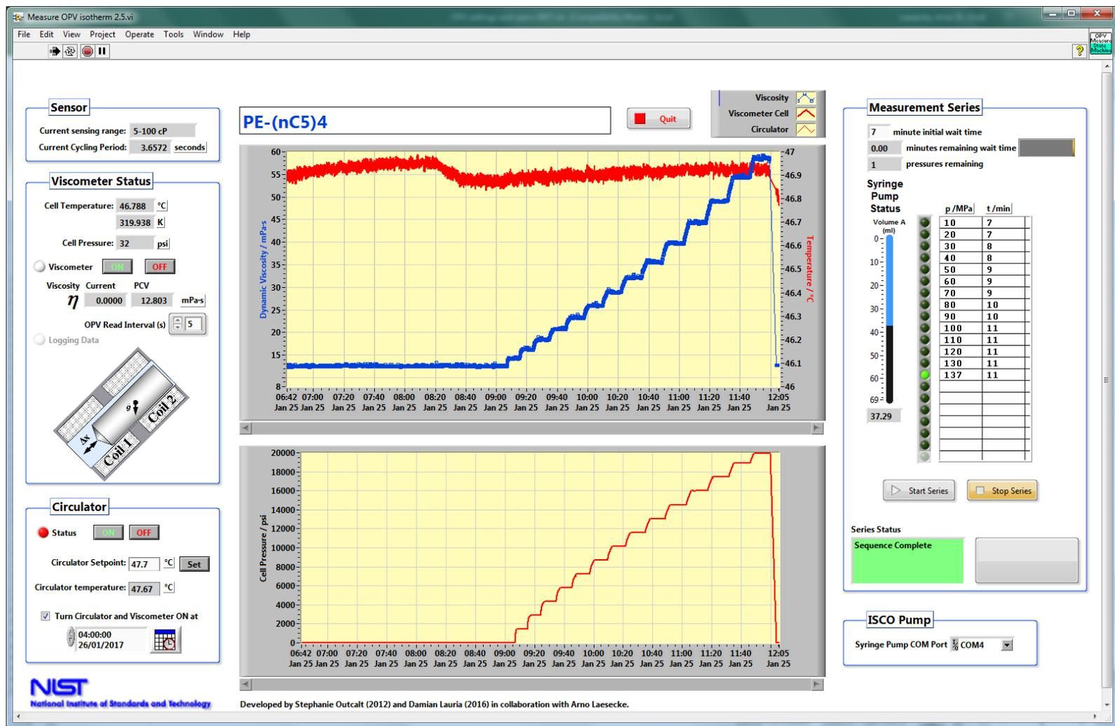
**Fig. 5.** Front panel of the custom LabVIEW virtual instrument (VI) developed in this project to automate the oscillating piston viscometer with the associated circulator and syringe pump for isothermal measurements over the entire pressure range. Features shown are traces of the cell temperature (red), the viscosity (blue), and the cell pressure (thin red) of the measurement of the POE-5 sample along the 320 K isotherm.
