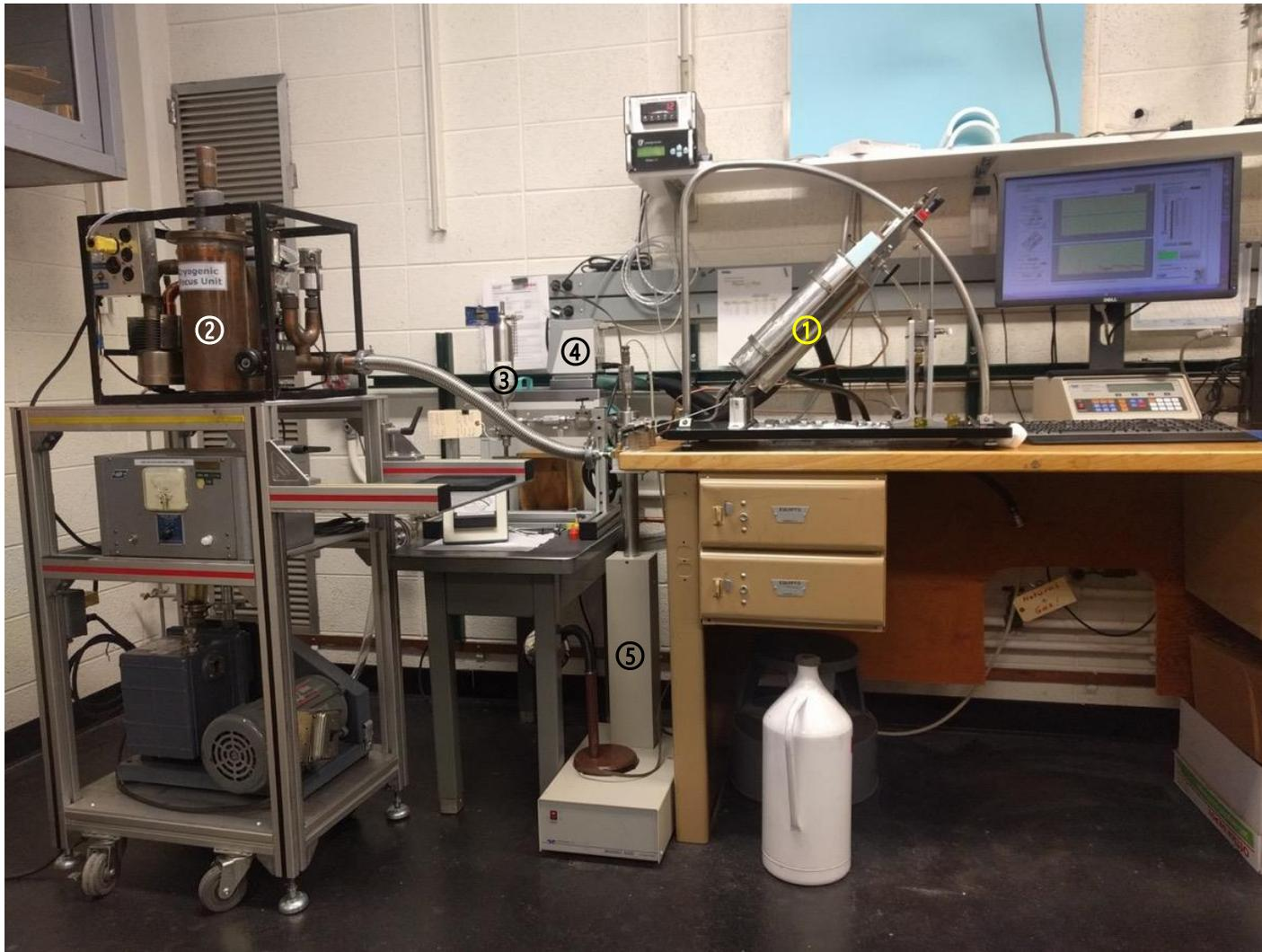
**Fig. 2.** View of the test stand with the oscillating piston viscometer (① above the drawers of the work bench) and the vacuum system ②, sample cylinder ③, circulator ④, and syringe pump ⑤.
