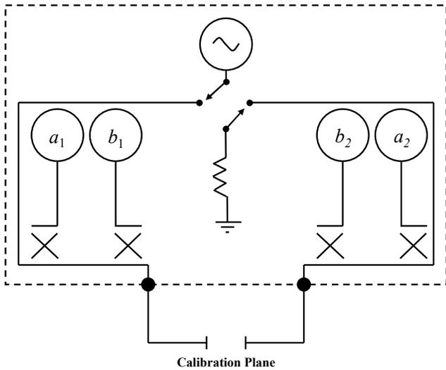
Fig. 1. Simplified schematic diagram of a four-sampler VNA.
