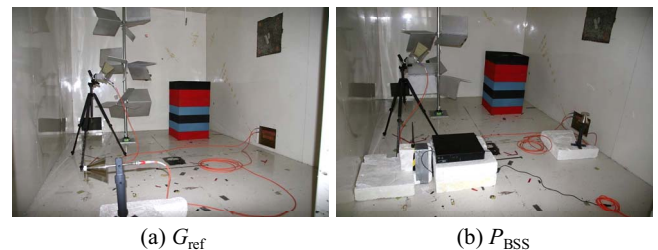
Fig 2: Photograph of set up shown in Fig. 1 for measuring (a) G_{ch} and (b) P_{BSS} . The absorbers are shown in the back, right corner of the chamber. The measurement antenna is on the tripod on the left, the reference antenna is shown in the front of (a) and on the right in (b), and the router is shown in (b).
