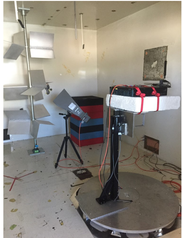
Fig. 4: Photograph of the automated setup for the reverberation chamber. The turntable has a translation stage for height adjustment and a platform with the router DUT attached by red straps.
