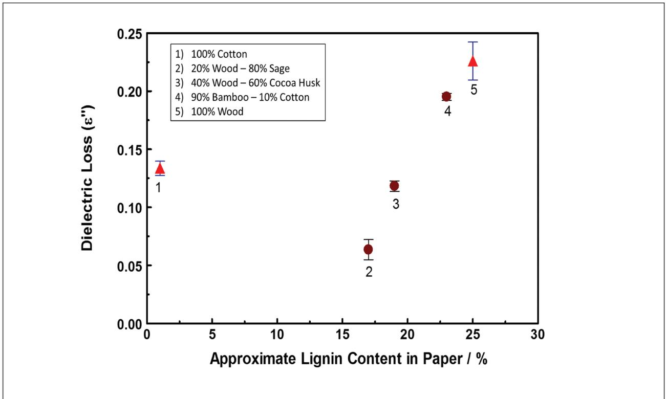
**1. Dependence of dielectric loss profiles (slope, see Eq. 1) on estimated weighted lignin fraction in the analyte. The weighted lignin fraction was calculated from the average literature values of lignin content in each fiber source weighted for the advertised composition.**
