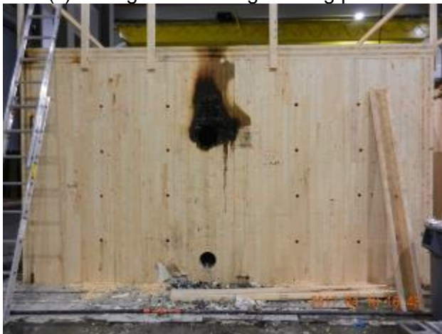
(e) drilled holes through wall panels
