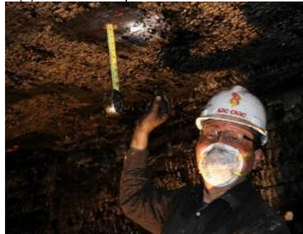
(d) char measurement by drilled holes
