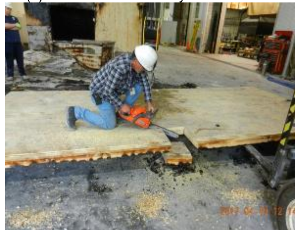
(f) cutting sample for char measurement
