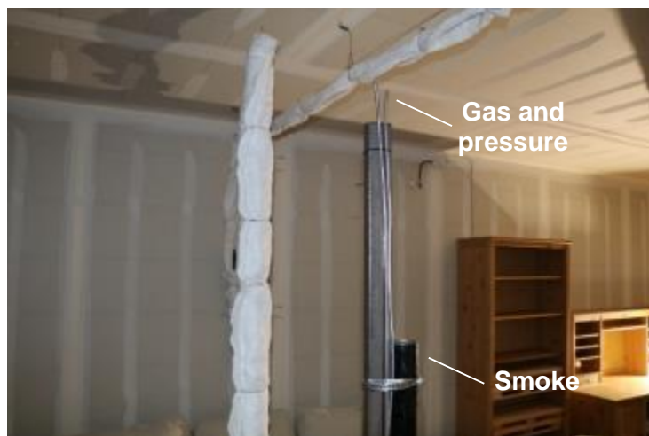
Figure 30. Photograph of stand with gas sampling tubes.
