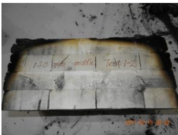
(c) middle block near TC Tree 6 charred 35 mm
