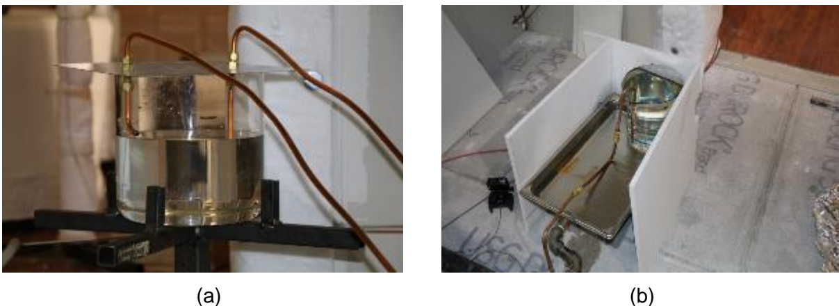
Figure 40. Photographs of water-cooled camera setup (a) 1 st attempt and (b) improved setup.
