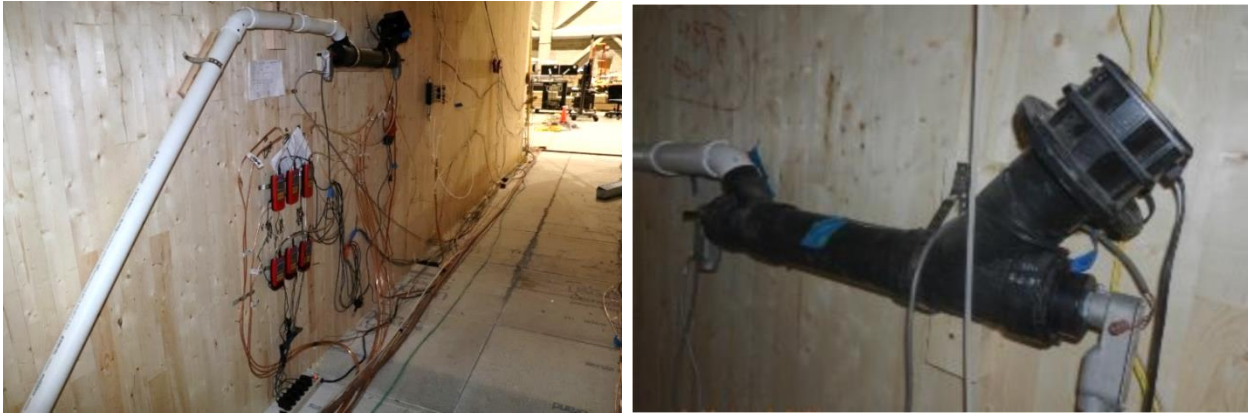
Figure 33. Photograph of smoke density meter (PVC pipe) and manometers mounted outside of the compartment.
