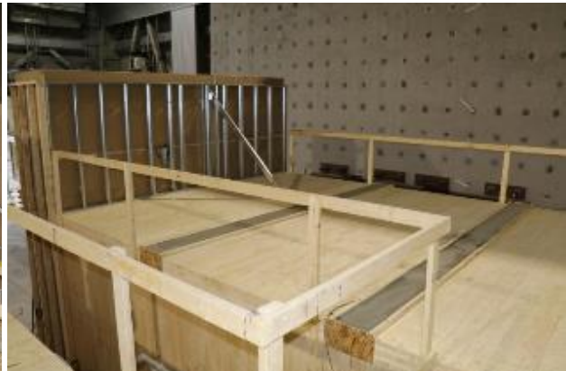
(b) gypsum concrete on top of ceiling joints
