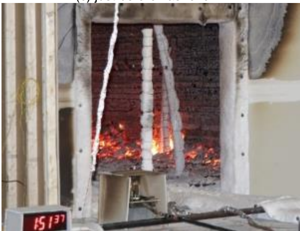
(e) exposed W1 wall at 111 min.
