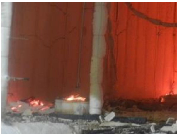
(a) CLT block near a TC Tree
