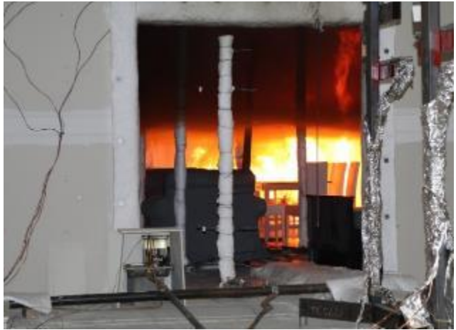
(b) W1 wall ignited at 9 min.
