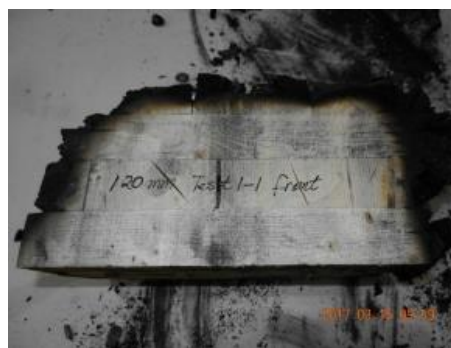
(b) front block near TC Tree 3 charred 55 mm
