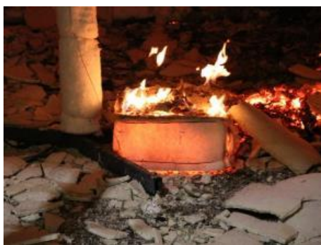
(a) CLT block near a TC Tree
