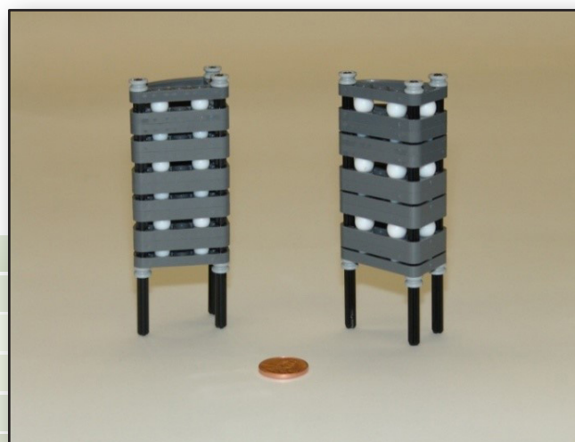
SRM 2087 Dimensional Standard for Medical Computed Topography
