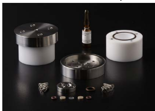
Figure 1: The prototype standard consists of a formalin ampule, a stainless-steel cap, a stainless-steel insert, two stainless steel frits with 2- \mu m pore size, a polydimethylsiloxane (PDMS) membrane, eight stainless steel screws, a PTFE base with 3 mL formalin well, and four o-rings.
