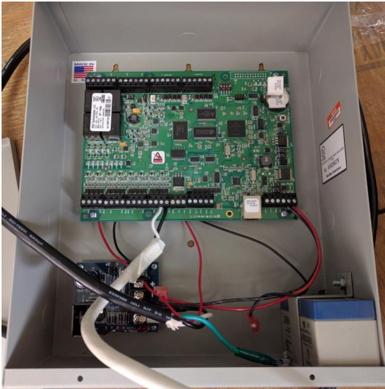
Figure 2-15 Inside of RS2 Door Controller Case
