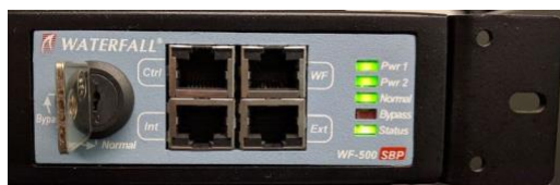
Figure 2-82 Waterfall Secure Bypass Interface
