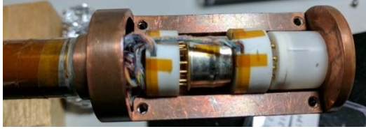
Fig. 1. Two QHR devices shown in the dual probe at AIST. One of the NIST graphene QHR devices is in the metal cap to the left and a AIST GaAs QHR device is in the plastic cap to the right. Both devices are mounted on TO-8 headers.
