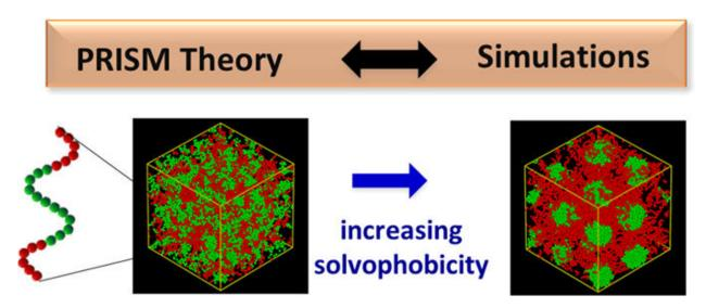
In this example, we use pyPRISM to predict the structure of amphiphilic block copolymer solutions. In this case, we show the impact of block copolymer sequence on self-assembly, in which the A block is hydrophilic and the B block is hydrophobic. The block sequences shown are A-B diblock (case 1), A-B-A triblock (case 2), and B-A-B triblock (case 2i), in which the fraction of A-block (f\_A) is always 0.5. The system and comparison data are taken from reference 1.
