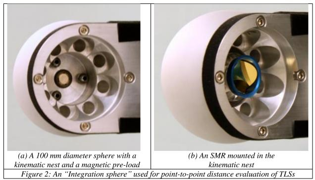
To enable a reference length measurement for the point-to-point distance tests (described in the later sections) a special custom sphere was commercially procured. This target, referred to
