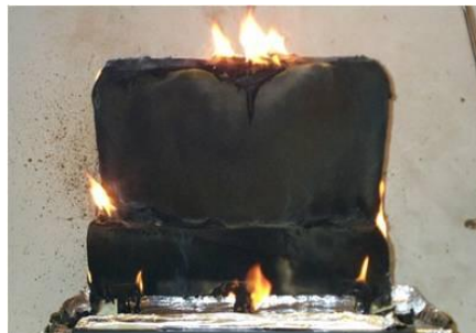
Barrier fabric test shows no flame penetration after six minutes. (Photo: NIST)
