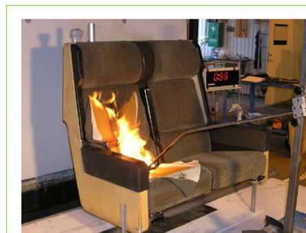
Fire testing of railcar passenger seats (Source: Lattimer’s presentation).
