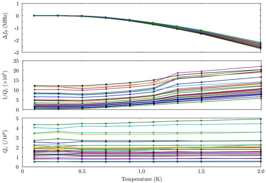
**Fig. 1** Resonance frequency shift, internal  $Q$  and coupling  $Q$  of several different resonators (each a different curve) as a function of temperature. These data were measured in an ADR and indicate that these important parameters can be measured at temperatures up to 500 mK without changing dramatically from their values at the lower temperatures used for readout scenarios (Color figure online)
