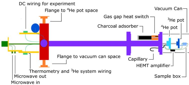
**Fig. 3** Diagram of the super rapid dip probe. A vacuum can enclose the  $^4\text{He}$  (1 K) pot, the  $^3\text{He}$  (300 mK) pot and the sample boxes, and the probe is submerged in liquid helium to a level somewhere above the capillary (Color figure online)
