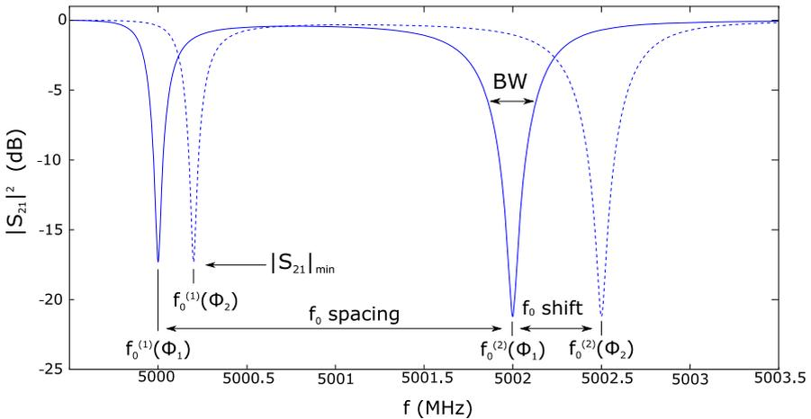
**Fig. 2** Model of an  $|S_{21}|$  measurement. The dashed line represents a measurement of the same two resonators with a different amount of flux ( $\Phi$ ) through the SQUIDs. Measurements are taken at approximately 20 different values of flux per resonator. This will provide the maximum  $f_0$  shift, and other parameters can be averaged over all of the flux points (Color figure online)
