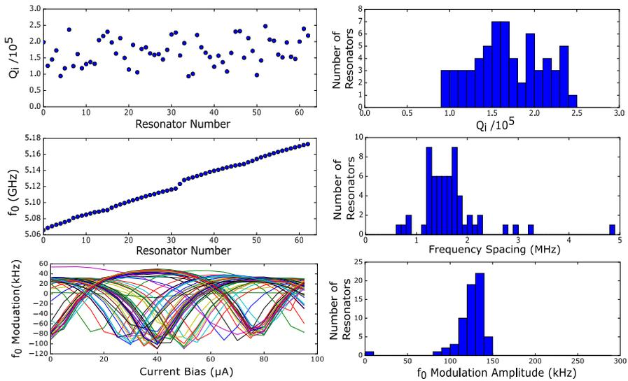
**Fig. 4** Data obtained from screening a 64-channel multiplexer chip. All data were obtained at 400 mK. One channel did not respond to flux through the SQUID, and one channel was not included in this survey because it was too close in frequency to another resonator (Color figure online)
