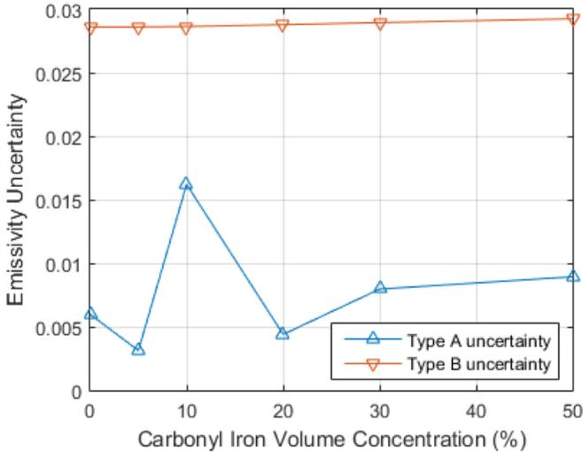
Fig. 6. Uncertainty contributions in thermal IR emissivity of epoxy-based microwave absorber material as a function of CIP loading concentration in percent tap volume.
