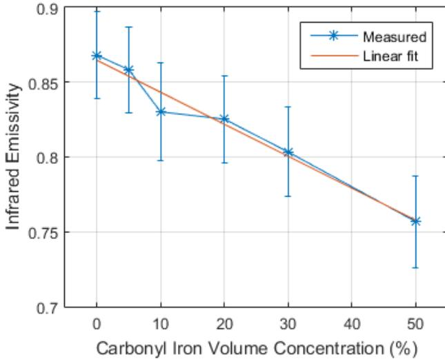
Fig. 5. Thermal IR emissivity of the epoxy-based microwave absorber material as a function of CIP loading concentration in percent tap volume. The blue line shows the measured data and the red line provides a linear fit of the data. Error bars are plotted as one standard uncertainty on either side of the data points.
