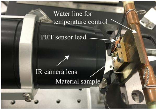
Fig. 1. Photograph of experimental setup for sample measurements.
