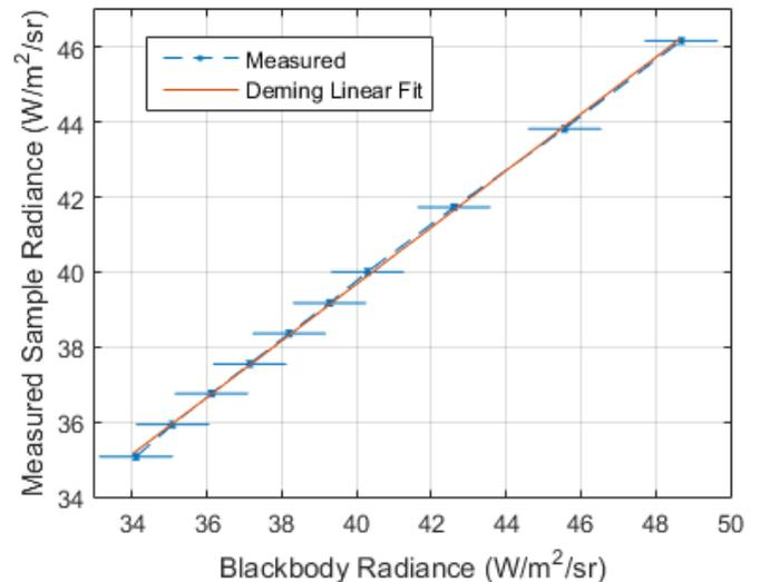
Fig. 4. Blue dashed line shows the measured IR radiance of the 50% CIP sample versus the measured blackbody radiance along with error bars in both the axes. Error bars are plotted as one standard uncertainty on either side of the data points. The red line shows the result of the Deming linear fit.
