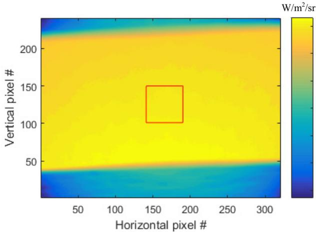
Fig. 2. Example of measured sample IR radiance image. The shown image is of the pure epoxy sample at a set temperature of 45 °C. The red box encloses the pixels used in the averaging.
