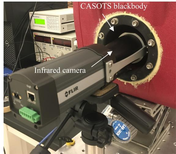
Fig. 3. Experimental setup for blackbody measurement. The IR camera looking into the CASOTS IR blackbody is shown.
