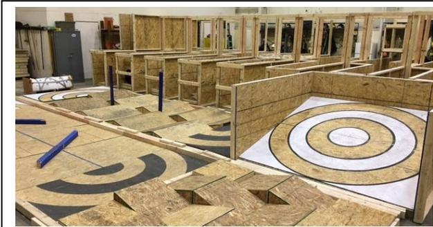
Figure 1: Ground robot tests for Operator Proficiency – Basic Skills at 120 cm (front) and 60 cm (rear) scales.
