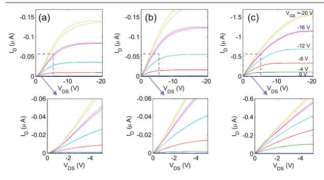
Figure 1: Changes to the ideality of I-V characteristics as a function of polymer ordering in three organic field effect transistors. As polymer ordering is increased from (a) to (c), current increases and low drain voltage characteristics become increasingly linear, and therefore closer to agreement with traditional field effect transistor characteristics.
