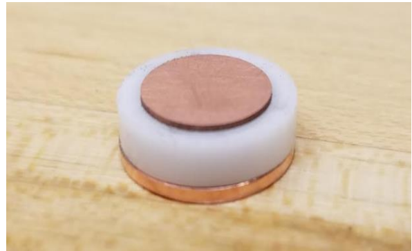
Figure 5: Powder filled copper and YSZ powder capsule
