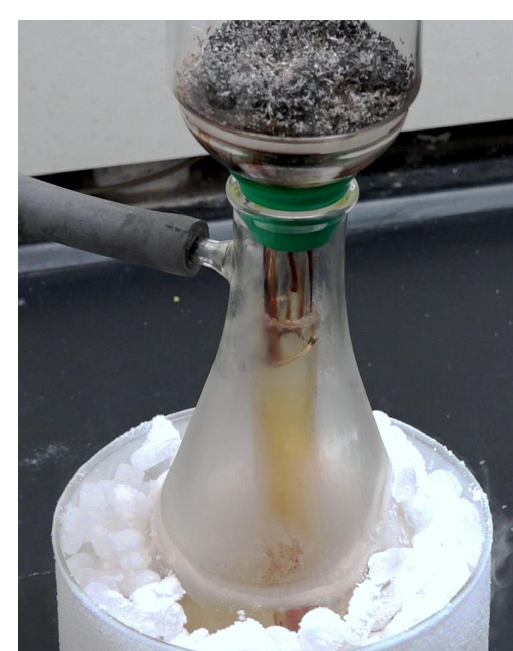
Figure 2: Photographs at different stages during the burning of SRM 3222 and smoke collection to produce the smoke condensate.
