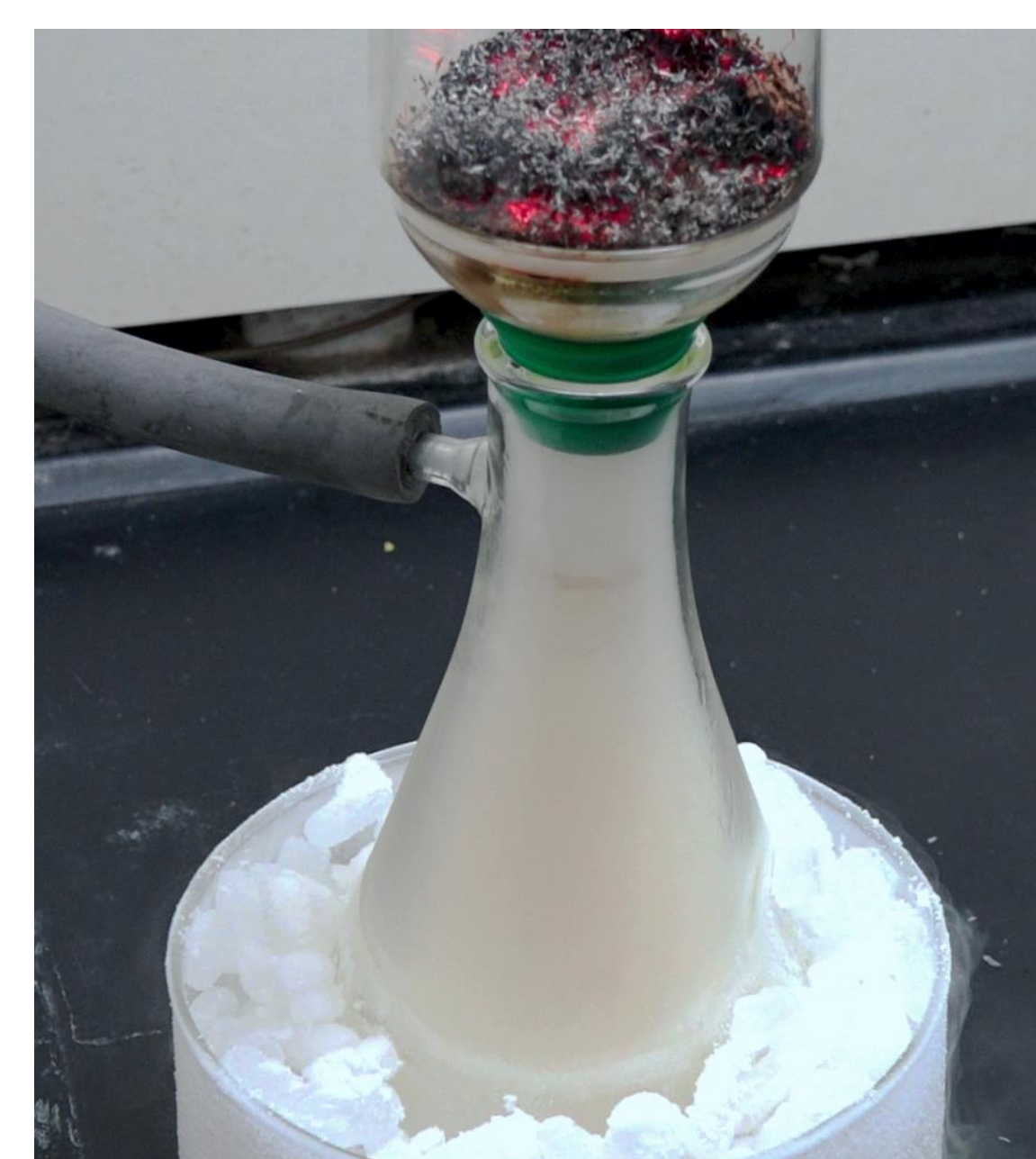
Figure 2: Photographs at different stages during the burning of SRM 3222 and smoke collection to produce the smoke condensate.
