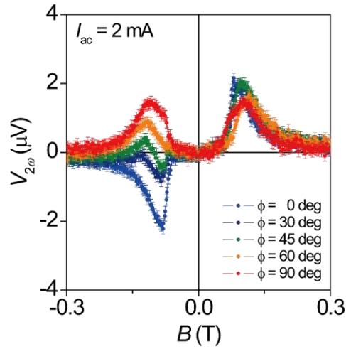
**Figure S6| Azimuthal angle-dependence of  $V_{2\omega}$  for Ti(2 nm)/NiFe(4 nm)/Ti(3 nm)/CoFeB(1.4 nm)/MgO sample.  $\phi = 0^\circ$  ( $90^\circ$ ) is for  $B=B_x$  ( $B_y$ ) representing damping (field)-like spin-orbit torque.**
