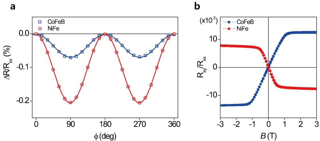
**Figure S5| Anisotropic magnetoresistance (AMR) and anomalous Hall resistance (AHE) of CoFeB(4 nm) and NiFe(4 nm) single layer samples. a,** AMR of CoFeB (blue symbols) and NiFe (red symbols). **b,** AHE of CoFeB (blue symbols) and NiFe (red symbols) structures.  $\phi$  is defined as an angle with respect to the current direction.
