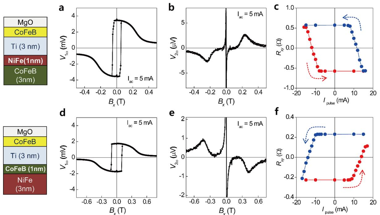
**Figure S7| The sign of spin-orbit torque in CoFeB/NiFe/Ti/CoFeB(perpendicular)/MgO (a, b, c) and NiFe/CoFeB/Ti/CoFeB(perpendicular)/MgO samples (d, e, f). First harmonic signals (a, d), second harmonic signals (b, e), spin-orbit torque switching data under  $B_x=10$  mT (c, f).**
