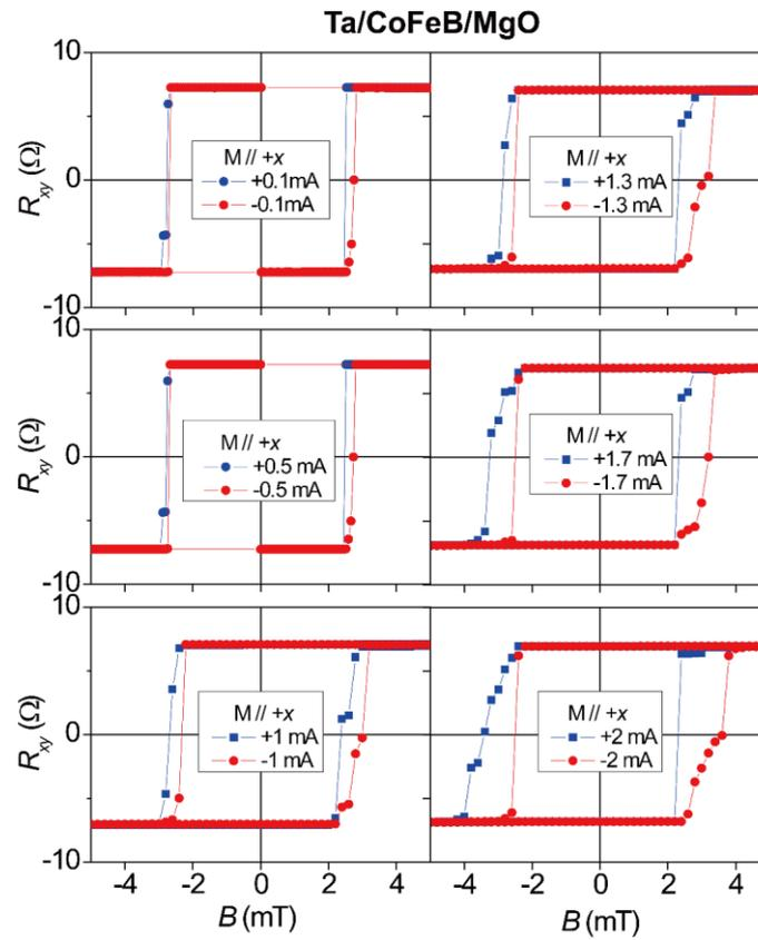
**Figure S8| Anomalous Hall resistance  $R_{xy}$  versus  $B_z$  curves with various d.c. currents in the presence of  $B_x$  for the Ta/CoFeB/MgO sample. The d.c. current ranges from 0.1 mA to 2 mA and  $B_x = +10$  mT.**
