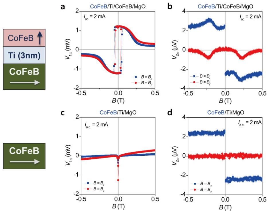
**Figure S2** | Raw data of the harmonic measurement for Ti(2 nm)/CoFeB(4 nm)/Ti(3 nm)/CoFeB(1 nm)/MgO and Ti(2 nm)/CoFeB(4 nm)/Ti(4 nm)/MgO samples. **a,b**, The first harmonic signal ( $V_{1\omega}$ ) (**a**) and second harmonic signal ( $V_{2\omega}$ ) (**b**) for the CoFeB/Ti/CoFeB/MgO structure. **c,d**,  $V_{1\omega}$  (**c**) and  $V_{2\omega}$  (**d**) for the CoFeB/Ti/MgO structure. The measurements are done with an a.c. current of 2 mA.
