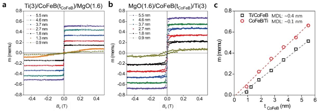
**Figure S1| Measurement of magnetic dead layer at Ti/CoFeB and CoFeB/Ti interfaces.**
