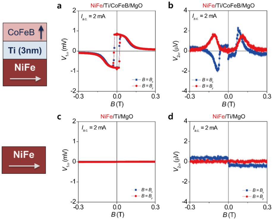
**Figure S3| Raw data of the harmonic measurement for Ti(2 nm)/NiFe(4 nm)/Ti(3 nm)/CoFeB(1.4 nm)/MgO and Ti(2 nm)/NiFe(4 nm)/Ti(4 nm)/MgO samples. a,b,** The first harmonic signal ( $V_{1\omega}$ ) (a) and second harmonic signal ( $V_{2\omega}$ ) (b) for the NiFe/Ti/CoFeB/MgO structure. **c,d,**  $V_{1\omega}$  (c) and  $V_{2\omega}$  (d) for the NiFe/Ti/MgO structure. The measurements are done with an a.c. current of 2 mA.
