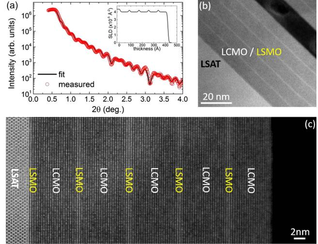
FIG. 1. (a) X-ray reflectivity data (red circles) and fit (black line) using GENX software [39] of the  $n = 2$  superlattice. Inset: Scattering length density profile obtained from the fit. (b) A low-magnification STEM HAADF image of the superlattice. (c) A high-magnification STEM HAADF image of the superlattice, viewed from the pseudocubic [110] direction.
