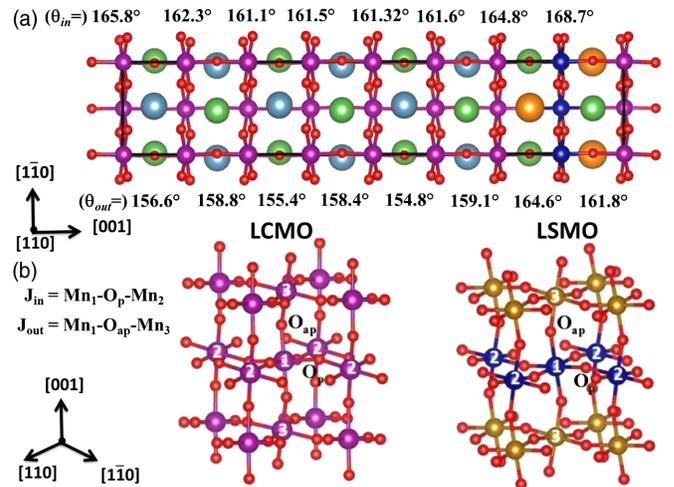
FIG. 3. (a) DFT-optimized structure of a  $(LSMO)_2/(LCMO)_6$  superlattice confirms the reduction of the octahedral rotations in the LSMO region. Here,  $\theta_{in}$  ( $\theta_{out}$ ) indicates the in-plane (out-of-plane) Mn—O—Mn bond angles. (b) In-plane  $J_{in}$  (via  $Mn_1$ -O<sub>p</sub>- $Mn_2$ ) and out-of-plane  $J_{out}$  (via  $Mn_1$ -O<sub>ap</sub>- $Mn_3$ ) nearest-neighbor isotropic exchange interactions shown for the LCMO and LSMO region.
