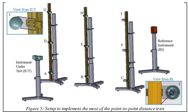
A test facility was set up at NIST to implement the procedures that could realize these tests. Per the proposed standard these tests can be implemented in any manner, but the setup depicted in Figure 5 was chosen to be implemented at NIST for the following reasons:
