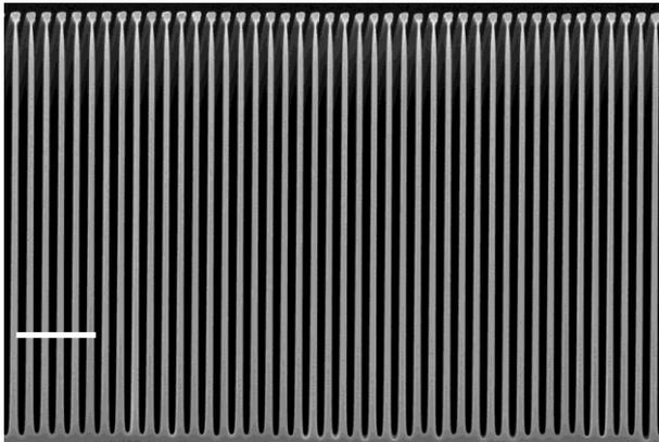
Fig. 2. Cross section SEM image of a 400 nm period grating etched to 10.6 μm via cryogenic process. Scale bar: 2 μm.
