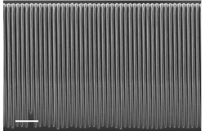
Fig. 3. Cross section SEM image of a 400 nm period grating etched to 11 μm via Bosch process. Scale bar: 2 μm.
