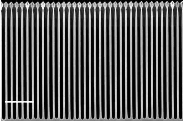
Fig. 1. Cross section SEM image of a 200 nm period grating etched to 4.4 μm via cryogenic process. Scale bar: 1 μm.
