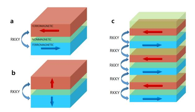
Figure: Schematic of synthetic antiferromagnets. a, bilayers with in-plane magnetization. b, bilayers with out-ofplane magnetizations. c, multilayers. The arrows within each ferromagnetic layer indicate the direction of magnetization. Depending on the magnetic configurations the RKKY coupling and dipolar fields add (a) or subtract
