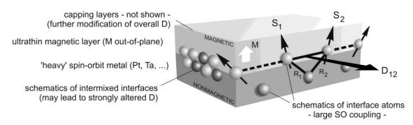
This interaction clearly favors a certain misaligned and turning sense (chirality) of the magnetic moments. Most important for magnetic multilayers are the DM interactions induced by interfaces between magnetic metals and metals with strong spin-orbit coupling. Figure adapted from Nature Nanotech. 8, 152 (2013).
