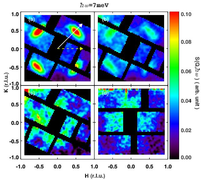
FIG. 1. (Color online) Inelastic neutron scattering measurements in the  $(HK0)$  plane measured on SEQUOIA at energy transfers  $\hbar\omega = 7$  meV from (a)-(c) SC40 and (d) Ni10 samples. The samples temperature are (a) 5 K, (b) 20 K, (c) 200 K and (d) 5 K. All slices were taken with an energy width of 2 meV. Intensity scale is the same in (a) to (c); data in (d) have been scaled to be directly comparable. Black regions of each panel represent gaps in the detector array.
