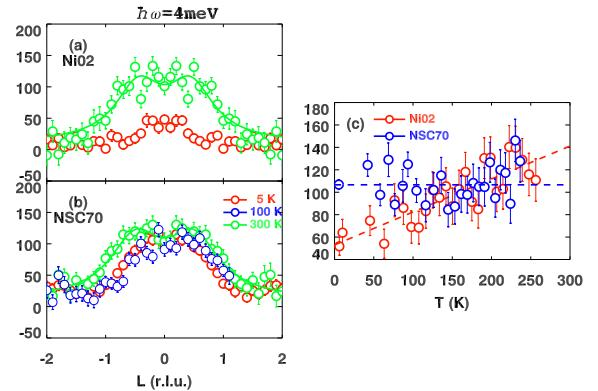
FIG. 4. (Color online) Inelastic neutron scattering measurements on (a) Ni02 and (b) NSC70 samples along  $(0.5, 0, L)$  at energy transfer  $\hbar\omega = 4$  meV, performed on BT7. The solid lines are fits to the two symmetric Lorentzian peaked at  $L = \pm 0.5$ . The intensities at  $(0.5, 0, 0.5)$  vs.  $T$  for both samples are plotted in (c). The dashed lines are guides to the eye. The error bars represent statistical error.
