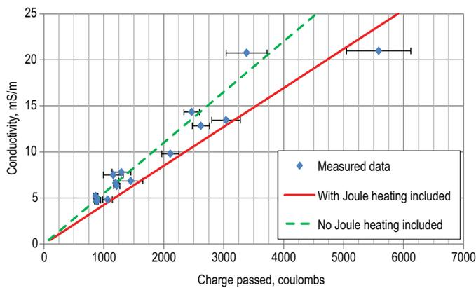
**Fig. 8: Calculated specimen conductivity as compared with cumulative charge passed for the 15 concrete mixtures. Diagonal lines indicate model relationships for calculations that are performed with and without the effects of Joule heating of the specimens being included.<sup>21</sup> Error bars indicate  $\pm$  one standard deviation in measured charge passed**
