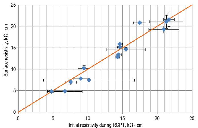
**Fig. 6: Measured surface resistivity as compared with resistivity calculated from initial current in the RCPT (both at 56 days) for the 15 concrete mixtures. The diagonal line indicates the expected one-to-one relationship. Error bars indicate  $\pm$  one standard deviation for the measured data**
