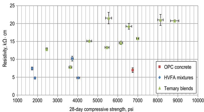
**Fig. 9: Surface resistivity (56 day) as a function of 28-day compressive strength for the 15 concrete mixtures. Error bars indicate  $\pm$  one standard deviation for the measured data (Note: 1000 psi = 6.9 MPa)**
