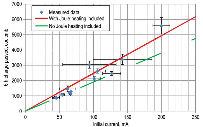
**Fig. 5: Measured cumulative charge passed over 6 hours (RCPT) as compared with measured initial current (both at 56 days) for the 15 concrete mixtures. Lines indicate conversion of initial current to cumulative charge passed with (current changes with temperature) and without (constant current) a Joule heating correction.<sup>18</sup> Error bars indicate  $\pm$  one standard deviation for the measured data**
