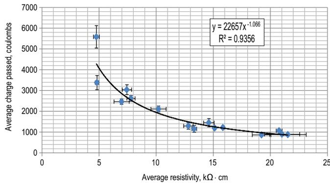
**Fig. 7: Average cumulative charge passed (RCPT) as a function of measured average surface resistivity at 56 days for the 15 concrete mixtures. Error bars indicate  $\pm$  one standard deviation for the measured data**
