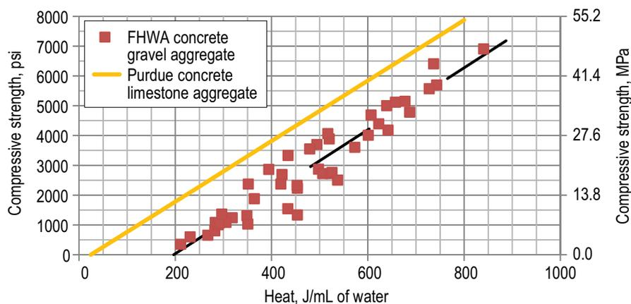
**Fig. 1: Measured compressive strength as a function of measured cumulative heat release (per unit volume of water). The strength-heat release relationship (dashed line) is a best-fit line used for adjusting mixture proportions. The relationship labeled as Purdue concrete is based on data from Reference 14**
