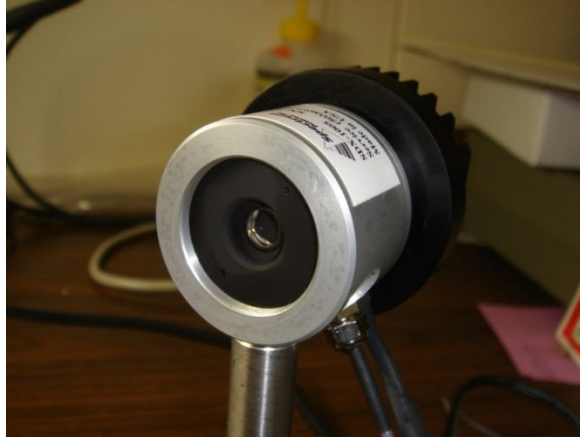
Fig. 2. Picture of a temperature controlled hybrid pyroelectric UV detector standard of low NEP. The LiTaO 3 crystal is covered with organic-black coating.
