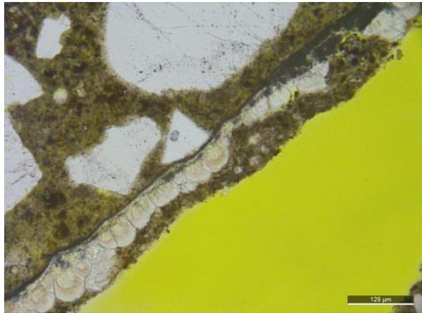
*Crack in the repair mortar*
