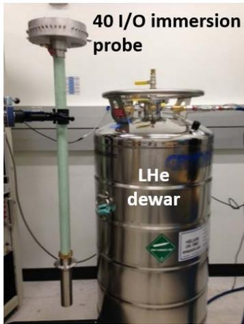
Fig. 3. NIST immersion probe with 40 input/output lines.
