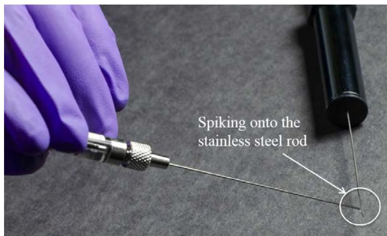
Figure 2. Illustration of direct loading of calibration liquid onto SPME stainless steel rod
