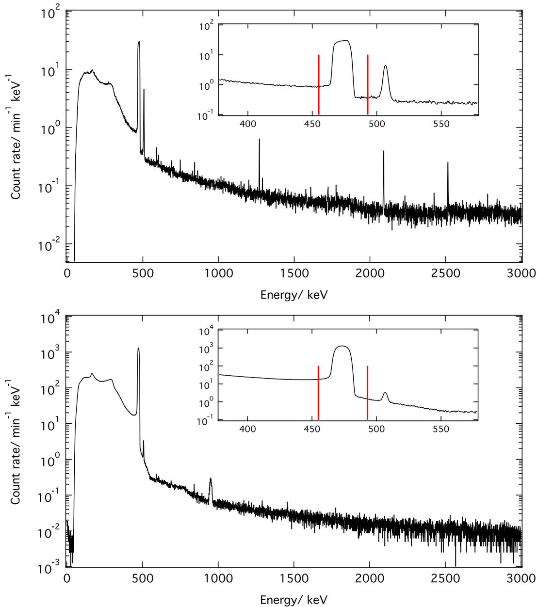
**Figure 8.** Top: plot of the gamma-ray spectrum from the thin <sup>10</sup>B target. The inset shows the region expanded around the 478 keV line, and the red lines indicate the analysis region. Bottom: plot of the gamma-ray spectrum from the thick <sup>10</sup>B target. The inset shows the region expanded around the 478 keV line, and the red lines indicate a typical analysis region.
