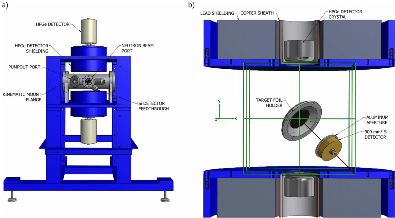
**Figure 1.** Illustrations of (a) the alpha–gamma device vacuum system (gray) in its support frame (blue) and (b) a section view of the alpha–gamma device showing the detection geometry; the neutron beam is incident on the target at the position of the green cross.
