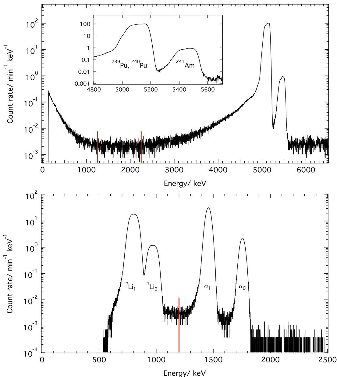
**Figure 7.** Top: charged particle spectrum from the  $^{239}\text{Pu}$  source. The inset indicates other isotopes that contribute to the alpha rate. The red lines indicate a typical region used for background subtraction. Bottom: charged particle spectrum from the thin  $^{10}\text{B}$  target. The red line indicates the position of a typical analysis threshold for counting the alpha particles.
