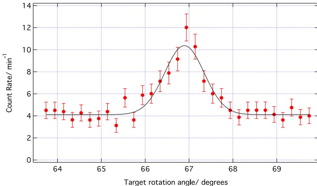
**Figure 16.** Plot of the measurement of the (101) reflection angle in the boron carbide target. The solid line is a fit to a Gaussian and flat background. The error bars represent statistical uncertainty only.
