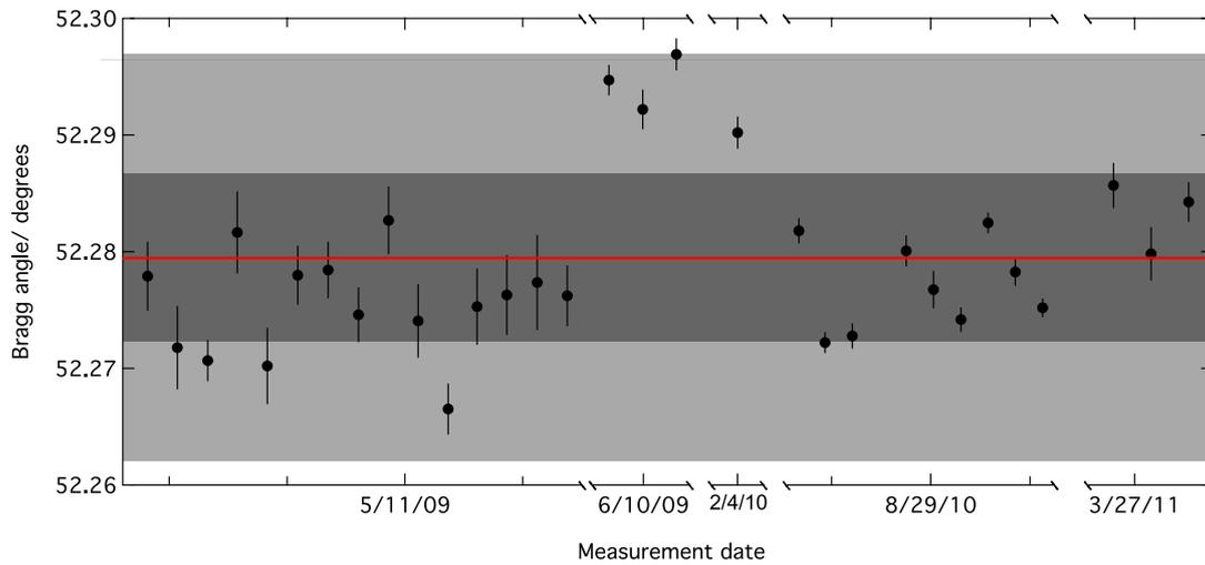
**Figure 13.** Plot of the measured  $\theta_{\text{Bragg}}$  angle. The centroid of the data (solid red line) is determined from a weighted constant fit ( $\chi^2/\text{d.o.f.} = 23.2$ ), and the dark shaded band corresponds to the  $\pm 1\text{-}\sigma$  uncertainty of that fit. The uncertainty used for the wavelength determination was conservatively chosen to include the entire data set and is denoted by the light shaded band.
