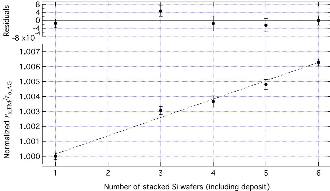
**Figure 21.** Measured ratio  $\frac{r_{\alpha,\text{FM}}}{r_{\alpha,\text{AG}}}$  as a function of the number of Si wafers stacked behind the monitor deposit. The dashed line is a linear fit, and the residuals are shown in the upper plot. The error bars represent statistical uncertainty only.
