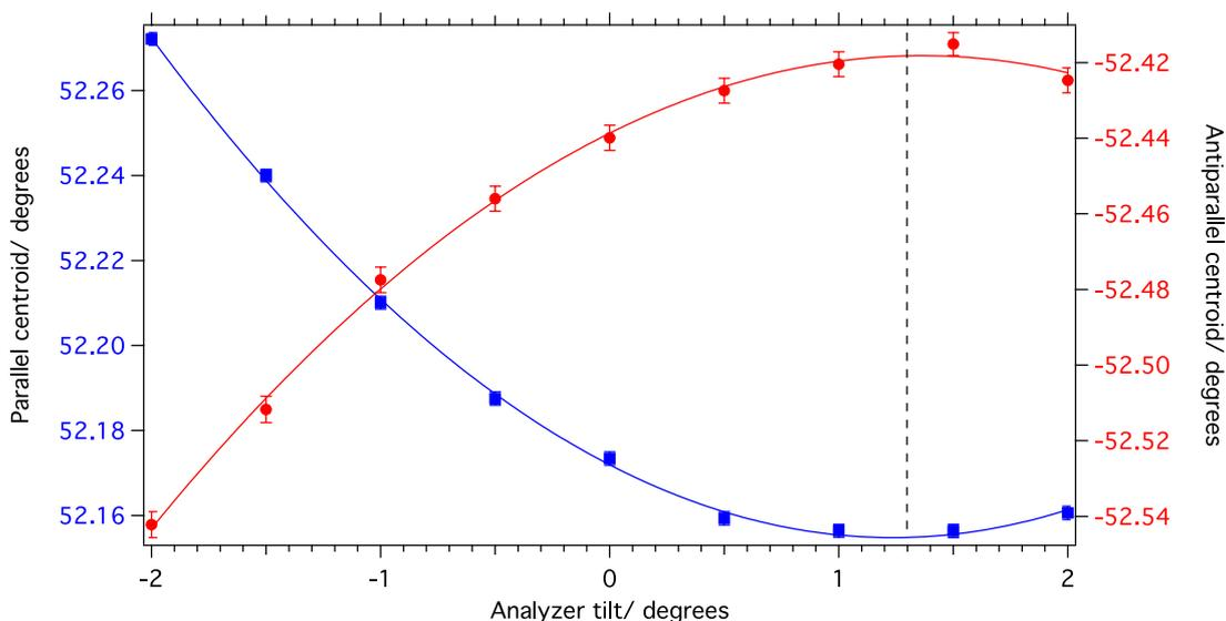
Figure 12. A tilt curve pair from the wavelength measuring apparatus. The solid lines are weighted fits to a parabola. The dashed line represents the tilt that best minimizes the parallel centroid and maximizes the antiparallel centroid. The error bars represent statistical uncertainty of the fit of the centroids.
