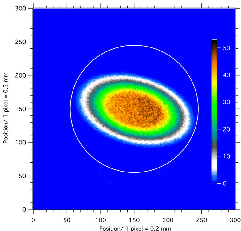
**Figure 14.** Beam images were acquired at the alpha–gamma deposit location with C1 = 15 mm and C2 = 7.2, 8.38, and 10.5 mm. The image for the largest collimation of C2 = 10.5 mm is shown here; the color scale represents linear intensity, and the image orientation is arbitrary. The white circle corresponds to the edge of the active area of the thin <sup>10</sup>B deposit.
