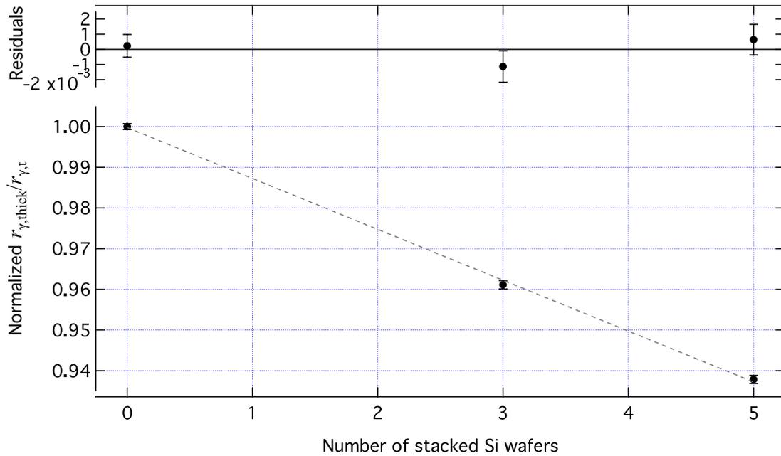
**Figure 15.** A plot of the ratio  $\frac{r_{\gamma,thick}}{r_{\gamma,t}}$  versus number of silicon wafers stacked behind the  $^{10}\text{B}$  target. A typical wafer is about 0.4 mm thick. The dashed line is a linear fit to the data; the residuals are shown in the upper plot. The error bars represent statistical uncertainty only.
