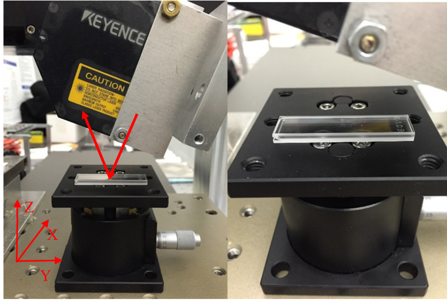
Figure 3. Triangulation probe setup for measuring a cuvette. The incident and reflected beam as a red line shows in the figure above.
