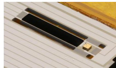
Figure 1. Photograph of a detector for space applications showing the nanotube forest on a silicon membrane.
