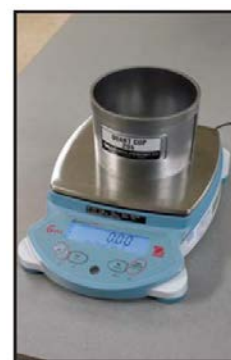
Figure 2. Zero weight of the empty quart kettle.
