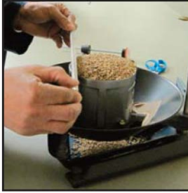
Figure 3a. Remove excess grain.
