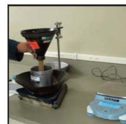
Figure 3. Filling the quart kettle from the filling hopper.
