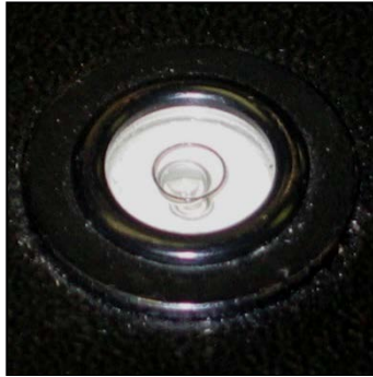
Figure 2-8. A Level Indicating Means Showing an In-level Condition.
