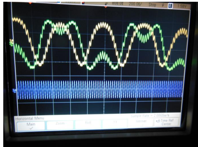
Figure 5. Photo-detector signals in quadrature with 1 kHz modulation on reference mirror. Blue (bottom) trace is accelerometer output.
