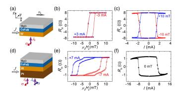
FIG. 1. Structures and current-induced switching behaviors in CoFeB with PMA, patterned with  $\alpha = 0^{\circ}$ . (a) Conventional SOT switching in W(1)/CoFeB(1)/MgO(1.8), (b) anomalous Hall effect (AHE) effect under +3 mA (blue solid circles) and -3 mA (open diamond circles), and (c) switching requiring a magnetic field. (d) Competing SOT effects of Pt/W/CoFeB/MgO. (e) AHE under positive and negative current. (f) Current induced magnetization switching requiring no magnetic field.
