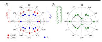
FIG. 4. Anisotropy of ZFS in Pt(3)/W(1.1)/CoFeB(1)/MgO(2) (in nm). (a) Angular dependence of the  $R_H$  values,  $I_C$ , and (b)  $\mu_0 H_{\perp}/J$  values, where the solid and open circles indicate magnetization switching from up to down and down to up, respectively.
