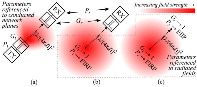
Fig. 1. An actual transmit system (a) and the “equivalent” radiator (b)-(c) excite plane waves with strength that is equal only along the dotted lines. The available output power from the actual receive antenna (a)-(b) is  $P_r$ ; the output power response of an isotropic antenna probe (c) given an equivalent incident plane wave is EIIP.
