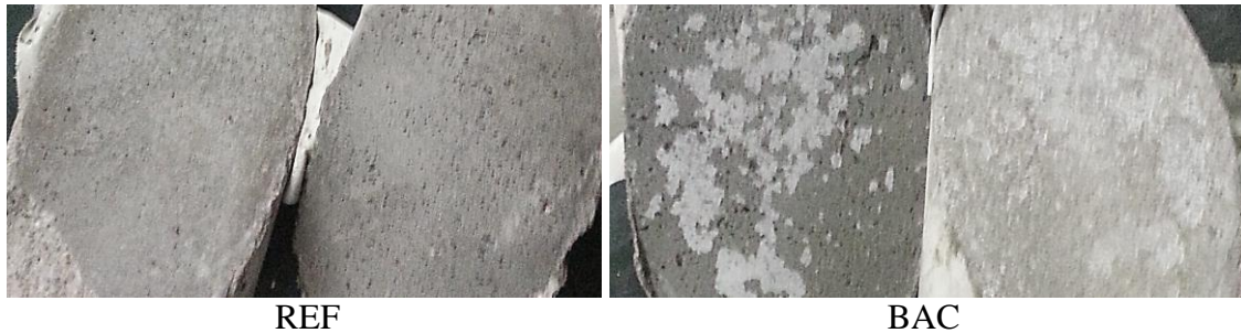
Figure 2: Bonding surfaces after performing the slant shear test
